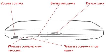
Figure 2-1 Front of the computer with display closed
